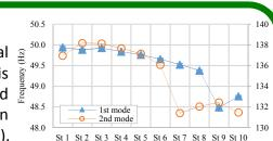
This is because the modal mass is relatively small compared to the first bending mode and making it more stiffness sensitive. On the other hand, the first mode appears to be creep sensitive (St.9-10).
