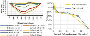
Performance is correlated to the cracks length and the profile deformations. Besides, each mode frequency seems to be more sensitive to different phenomena (stiffness, irreversible creep, etc.).
